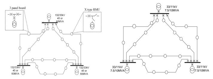
With higher utilisation factors incremental load growth can be absorbed more efficiently before reinforcement is triggered. When the group load reaches its maximum then a further transformer can be simply added or 'plugged in' to the network or the transformer group can be reconfigured by the movement of network split points.
