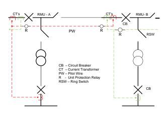
A simplistic illustration of unit protection as applied to the SP Manweb urban network is shown opposite purely to illustrate the additional components required over and above those employed in traditional network designs.
